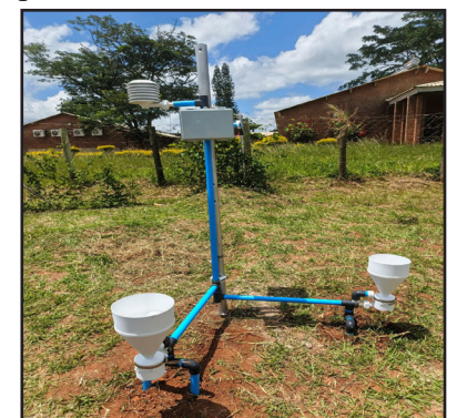
A 3D-Printed Automatic Weather Station developed by DCCMS staff and installed at Bvumbwe Meteorological Station.
